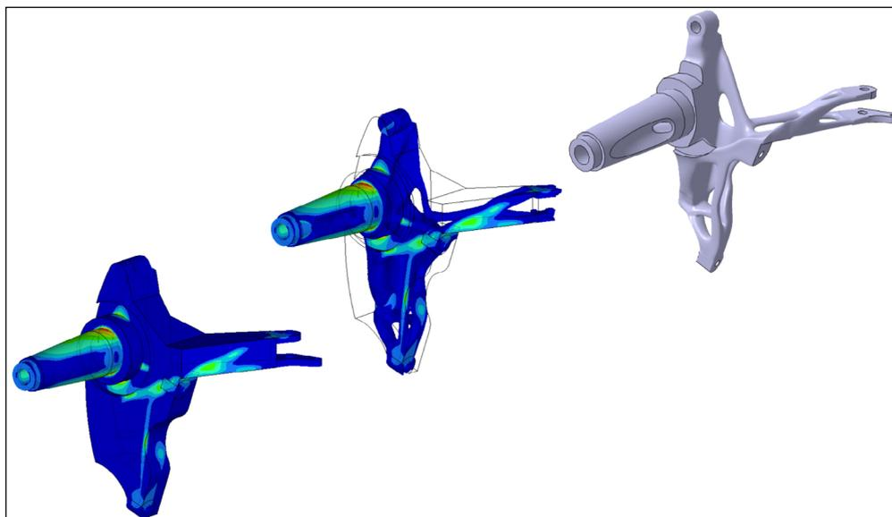
Finite element analysis of the start design of a wheel bearing technology demonstrator (left); numerical design optimization of the technology demonstrator to reduce the component's mass without impairing functionality (center); and CAD template for manufacturing the 3D metal component (right). © Fraunhofer EMI | Picture in color and printing quality: [www.fraunhofer.de/en/press](http://www.fraunhofer.de/en/press)
