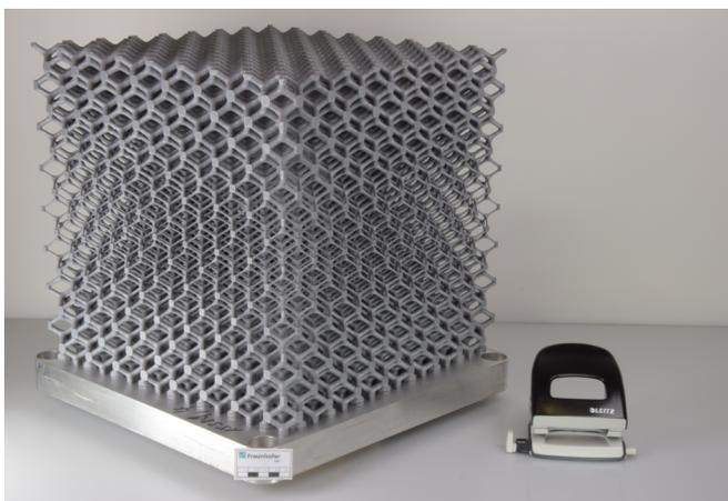
**Lattice cube with edge length of 40 centimeters, one of the largest metal structures manufactured using selective laser melting (SLM). © Fraunhofer EMI | Picture in color and printing quality: [www.fraunhofer.de/en/press](http://www.fraunhofer.de/en/press)**
