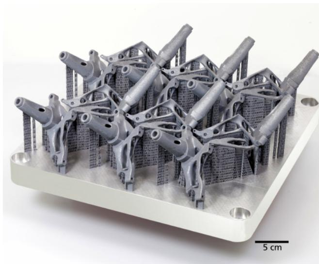
Several structural components arranged on a base plate after a selective laser melting process. © Fraunhofer EMI | Picture in color and printing quality: [www.fraunhofer.de/en/press](http://www.fraunhofer.de/en/press)
